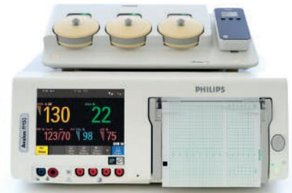
Avalon Smart Pulse provides a basis for confident decision making. Its integrated sensors emit infrared light that is invisible to the human eye, but reflected by tissue and blood vessels. The pulsating diameter of the small arteries causes changes in the reflected light. These changes are then measured and evaluated in an algorithm which then displays a maternal pulse value.
